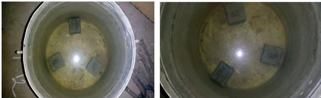
**Figure4.** Sample subjected to water absorption
